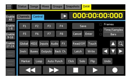
IMPORTANT NOTE: When using Studio One, the control surface must be turned on and configured before Studio One software is started. This is because setup information isn't sent after the program has been launched.
