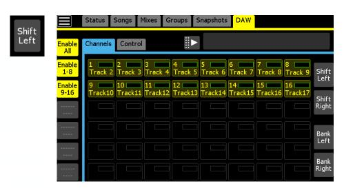
The channels in the configuration below have been "shifted" right by one.
