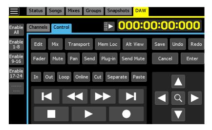
The Mackie HUI: Pro Tools Control tab contains HUI controls that operate as they do on a Mackie HUI control surface and are labeled for their specific functions in Pro Tools. All Pro Tools meter modes display correctly in the TC display.
