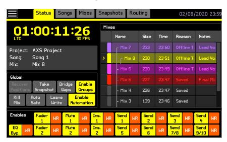
NOTE: Vision consoles have additional function enables that support Aux Send On/off and EQ Bypass. DAW enables are also available from the Vision Status page.
