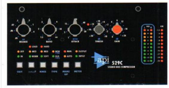
The centre section includes space at the top for the excellent optional 529C Stereo Bus Compressor which includes most of the features of the much-loved 2500 compressor. The Aux send and Summing Bus masters include Solo buttons and other useful routing tricks, particularly helpful for surround use. You can select External inputs for the sends, and individually insert Talkback.
