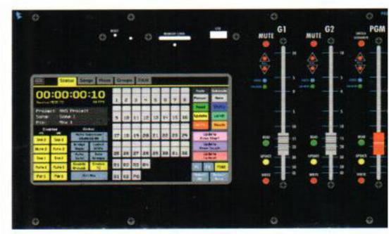
Program master which is attenuation only, with OdB at the top. It is worth noting that Final Touch can be added at a later date as an upgrade to a 2448 that is initially supplied without automation.
