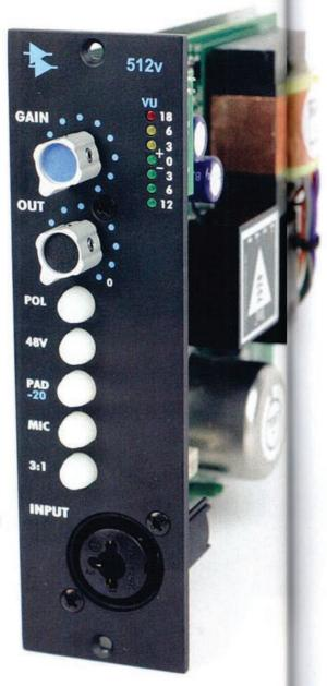
rack, I set about lining up the 512v. OVU on its LED meter (which meters the post-gain input level) gave me -18dBFS on the meter of my MOTU 896, with the detented output attenuation control in the two o'clock position. Turning that control clockwise to zero attenuation added a further 6dBFS to the output level. Turn it fully anti-clockwise and, as you might expect, the 512v's output level is reduced to zero.
