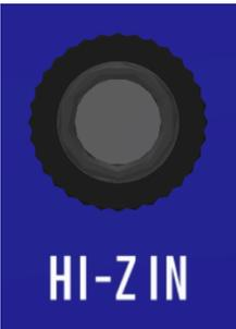
**HI-Z IN:** High-impedance, 500k $\Omega$ , unbalanced instrument input
