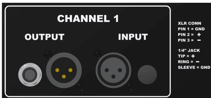
*IMPORTANT NOTE: Care should be taken not to short the outputs, as damage will occur to the output stage.*
