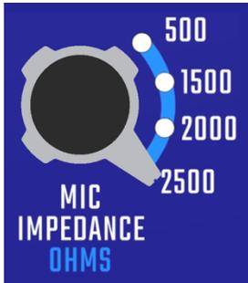
**MIC IMPEDANCE OHMS:** Selects the impedance of the microphone INPUT
