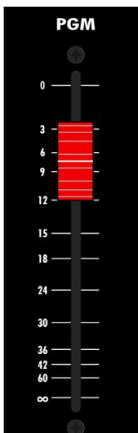
The fader with the red fader cap below the master section is the stereo program master fader. The master fader handles the left and right program bus audio on a single stereo fader.
