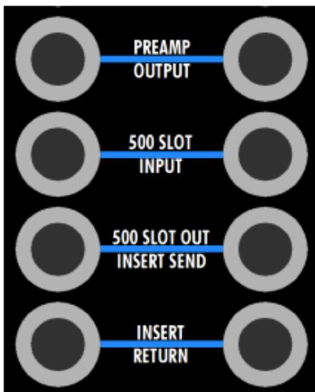
PREAMP OUTPUT: ¼” tip-ring-sleeve, balanced, low-impedance, line-level
