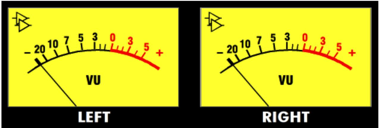
The meters are fed from the C/R SOURCE selectors above the control room monitors controls.
