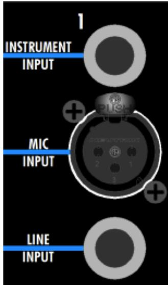
**INSTRUMENT INPUT:** ¼” tip-sleeve, unbalanced, high-impedance
