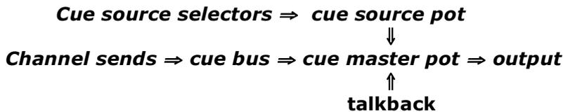
The stereo cue bus is the primary source for the cue master. Additional stereo sources can be added using the CUE SOURCE selectors and level control. Sources are selected using the CUE SOURCE switches. The level of the selected sources feeding the CUE MASTER is controlled by the CUE SOURCE potentiometer. The CUE MASTER potentiometer is fed from the cue bus and the CUE SOURCE pot and controls the overall output of the cue system.
