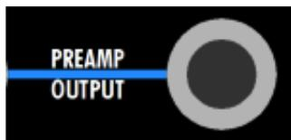
**PREAMP OUTPUT:** ¼” tip-ring-sleeve, balanced, low-impedance, line-level
