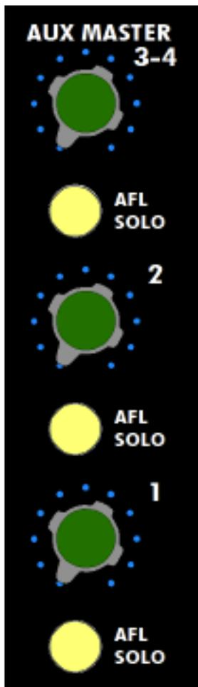
AUX MASTER 3-4: Output level control for auxiliary buses 3 and 4
