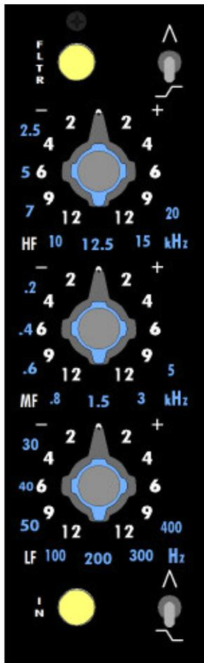
The API 550A Equalizer provides three (3) bands of equalization and a band-pass filter. It has been slightly repackaged for installation on input channels 1-2. Other than the repositioning of some controls these equalizers are identical to other 550A EQs.
