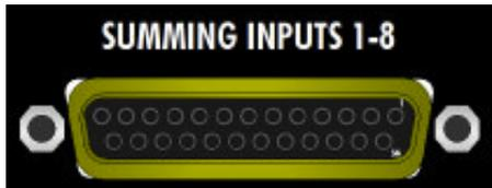
SUMMING INPUTS 1-8: DB-25, balanced, low-impedance, line-level
