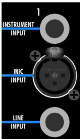
INSTRUMENT INPUT: 1/4" tip-sleeve, unbalanced, high-impedance
