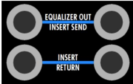
EQUALIZER OUT- INSERT SEND: ¼” tip-ring-sleeve, balanced, low-impedance, line-level
