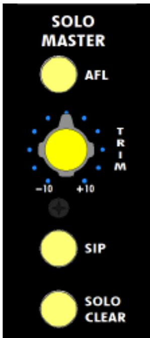
AFL (after-fader-listen): Enables the after-fader-listen solo mode
