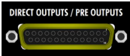
The DIRECT OUTPUTS / PRE OUTPUTS connector carries direct or preamp outputs from input channels 1-4, as well as the insert send from input channels 1 & 2 and the preamp outputs from input channels 3 & 4.
