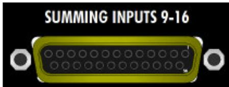
SUMMING INPUTS 9-16: DB-25, balanced, low-impedance, line-level
