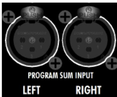
PROGRAM SUM INPUT (LEFT & RIGHT): 3-pin female XLR, balanced, low-impedance, line-level
