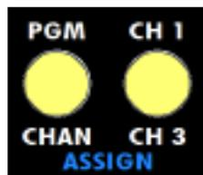
Assignments to input channels are accomplished using the two ASSIGN switches on the compressors. Engaging the PGM-CHAN switch will move the compressor from the program bus to the input channels. When PGM-CHAN is engaged, compressor 1 is assigned to input channel 1 and compressor 2 is assigned to input channel 2 by default. Engaging CH 3 or CH 4 assigns the compressors to these channels. These switches illuminate when engaged.
