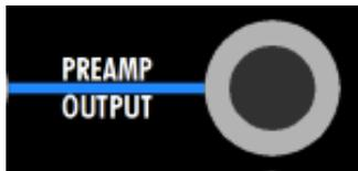
**PREAMP OUTPUT:** 1/4” tip-ring-sleeve, balanced, low-impedance, line-level
