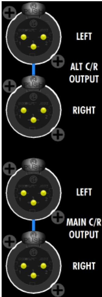
ALT C/R OUTPUT (alternate control room outputs): 3-pin male XLR, balanced, low-impedance, line-level
