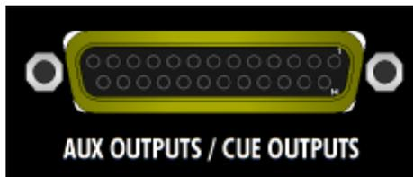
**AUX OUTPUTS / CUE OUTPUTS:** DB-25, balanced, low-impedance, line-level
