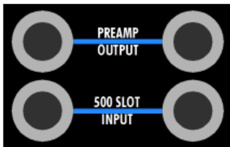
PREAMP OUTPUT: ¼” tip-ring-sleeve, jack\* balanced, low-impedance, line-level
