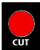
CUT: Mutes the selected control room loudspeakers when engaged
