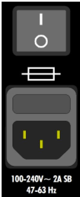
POWER SWITCH: On/off AC power switch
