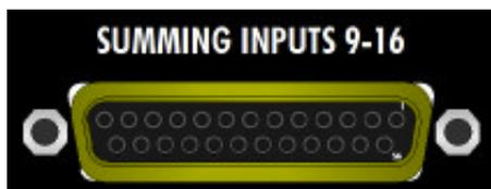
SUMMING INPUTS 9-16: DB-25, balanced, low-impedance, line-level
