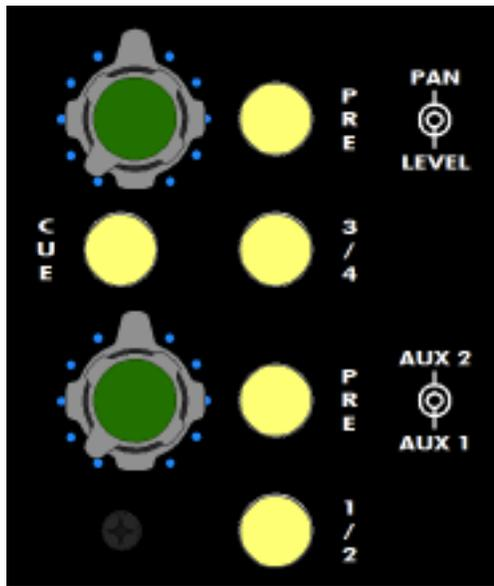
“The BOX” is equipped with four (4) auxiliary sends fed by two (2) mono auxiliary sends (1/2), and one (1) stereo auxiliary/cue send (3/4).
