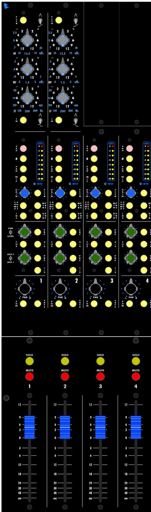
“The BOX” provides four (4) input channels that are designed primarily for recording, but can be used as additional channels while mixing.
