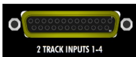
2 TRACK INPUTS 1-4: DB-25, balanced, low-impedance, line-level
