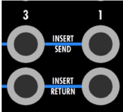
INSERT SEND: ¼” tip-ring-sleeve, balanced, low-impedance, line-level
