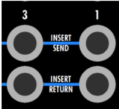
EQUALIZER OUT- INSERT SEND: ¼” tip-ring-sleeve, balanced, low-impedance, line-level
