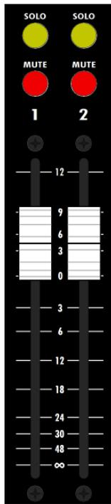
The fader modules with white fader caps contain the faders, MUTE and SOLO switches for summing inputs 1-16 (1 & 2 shown). The summing input fader controls for each pair of channels are arranged in a side-by-side configuration.
