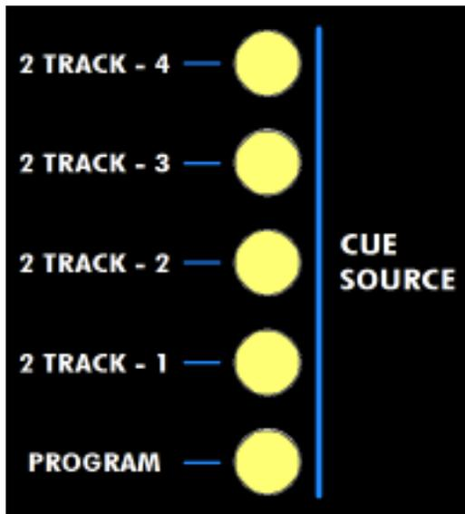
In addition to the stereo cue bus, the C/R SOURCE selections (PROGRAM\*) and up to four (4) external stereo sources can be routed to the cue master. These additional cue sources are selected using the CUE SOURCE selector switches and routed to the cue master via CUE SOURCE level control.
