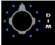
DIM: Sets the control room loudspeaker DIM level
