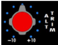
ALT TRIM (alternate trim): Trims the alternate control room loudspeaker outputs
