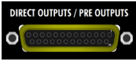
The DIRECT OUTPUTS / PRE OUTPUTS connector carries direct or preamp outputs from input channels 1-4, as well as the insert send from input channels 1 & 2 and the preamp outputs from input channels 3 & 4.
