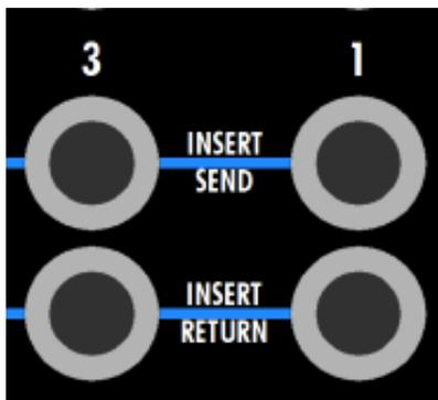
INSERT SEND: ¼” tip-ring-sleeve, balanced, low-impedance, line-level
