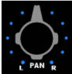
PAN (pan-pot): Continuously variable left-right stereo pan-pot
