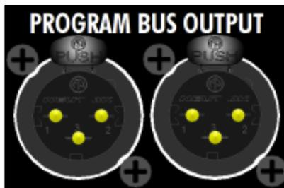
PROGRAM BUS OUTPUT (LEFT & RIGHT): 3-pin male XLR, balanced, low-impedance, line-level
