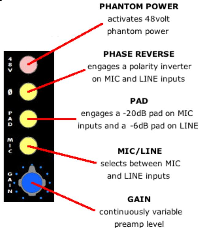
No switches engaged: LINE INPUT is selected by default
