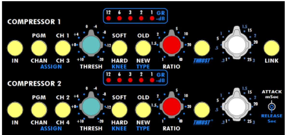
To use the compressors while mixing, they need to be assigned to the program bus, with Compressor 1 assigned to Left side of the program bus and Compressor 2 assigned to the Right. The compressors are located after the PROGRAM SUM INPUT and pre-insert.
