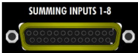
SUMMING INPUTS 1-8: DB-25, balanced, low-impedance, line-level
