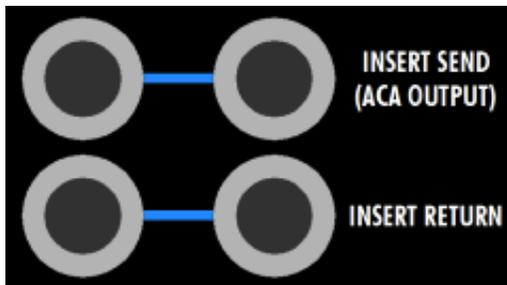
INSERT SEND (ACA OUTPUT) (LEFT & RIGHT): ¼” tip-ring-sleeve, balanced, low-impedance, line-level
