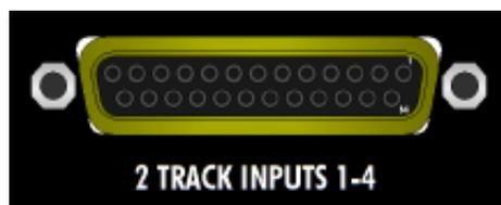
2 TRACK INPUTS 1-4: DB-25, balanced, low-impedance, line-level
