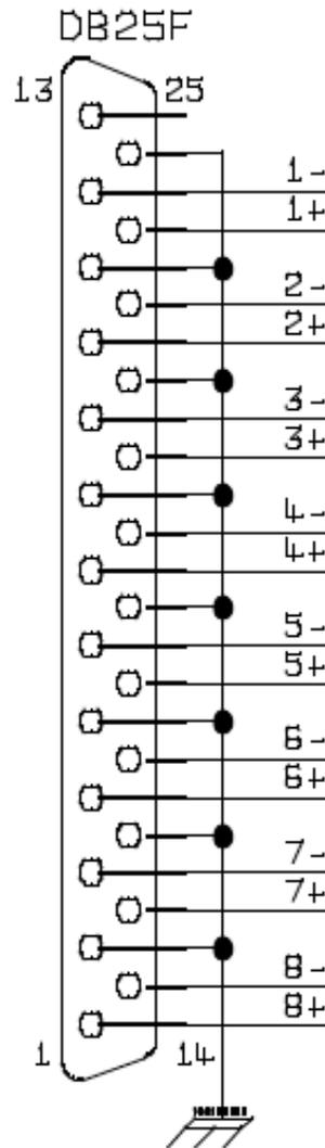
**Summing Input Line Input Connections**
