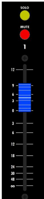
The fader module with blue fader caps contains the faders, MUTE and SOLO switches for input channels 1-4. These faders are the primary output level controls for the input channels.
