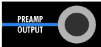
PREAMP OUTPUT: ¼” tip-ring-sleeve, balanced, low-impedance, line-level
