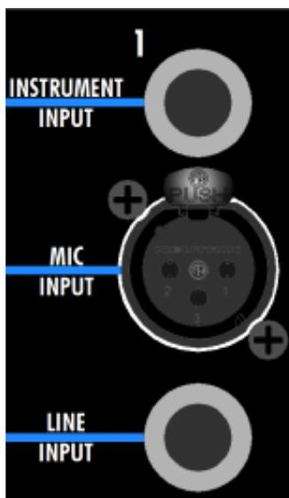
**INSTRUMENT INPUT:** ¼” tip-ring-sleeve, unbalanced, high-impedance
