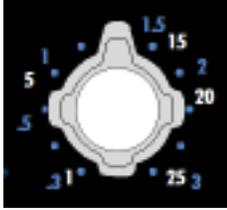
Attack and release times are fully variable on the 527 compressor and share a dual-concentric potentiometer for control. Attack time is adjusted using the outer ring of the pot and Release time is adjusted using the inner knob.
